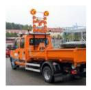
**LIGHT ARROW SS15 WITH VHS-2** SUPPLIED FROM BATTERY 12V/18OAH KEEPS FLASHING NONSTOP FOR UP TO 25 HOURS
