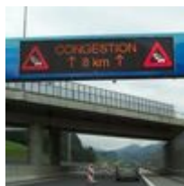
Variable message signs VMS LED
