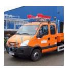
LIGHT ARROW SS15 LED WITH VLS-2 SUPPLIED FROM BATTERY 12V/18OAH KEEP FLASHING NONSTOP FOR UP TO 6 DAYS
