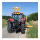
LIGHT ARROW SS15 LED SUPPLIED FROM BATTERY 12V/18OAH KEEPS **FLASHING NONSTOP FOR UP TO 11** DAYS
